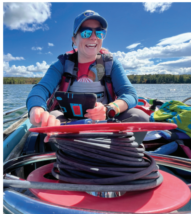
Assistant Lake Scientist Lizzy Gallagher lowers a probe to measure water temperature and oxygen levels while collecting water samples in October. 7 Lakes collects and analyzes samples throughout the fall to determine when a lake's water "turns over" after being stratified by temperature throughout the summer.
