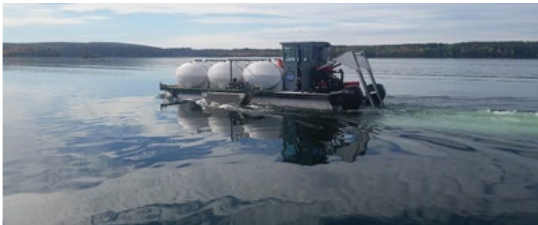
Alum (aluminum sulfate) carefully applied in East Pond by SOLitude barge
