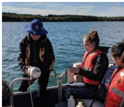
Students and staff from Colby College monitor alum distribution and pH levels to ensure that the correct dose of alum is administered. The students documented that the alum contractor kept pH at between 6.5 and 7.5 to prevent harm to fish and other aquatic life.
