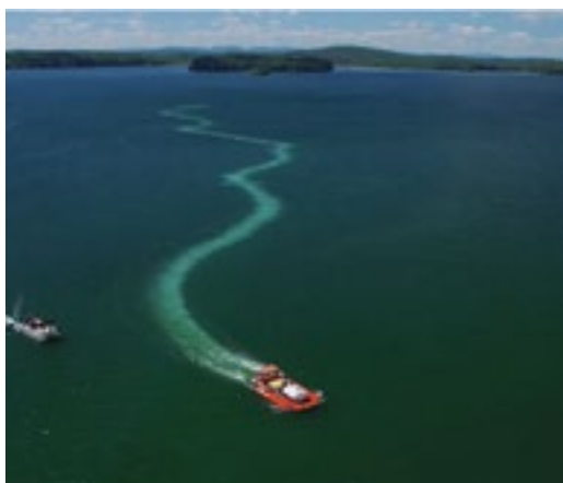
Alum falls to the lake bottom where it binds with phosphorus-rich sediment, preventing it from feeding summer algae.
