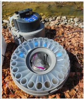
Stream sites around North Pond, autosampler, and bottles after a rain event.
